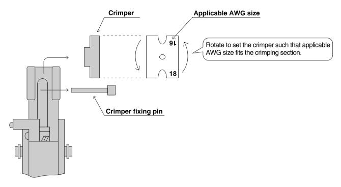
[Manual crimping tool : crimped section]
